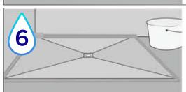
Tape all the joints between shower tray, wall and floor using Mira Safecoat Roll and Mira Multicoat 4400.
